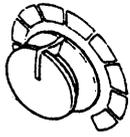
The dial adjusts generator output voltage.
