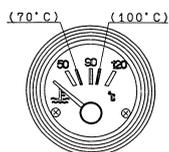
Water Temperature Gauge displays the temperature of engine coolant. Normal temperature may vary depending on the environment, but it should be between 75 to 90 degrees Celsius.
