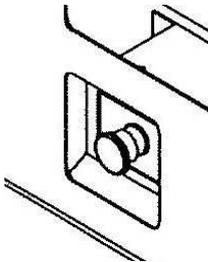
This button is used to stop the engine in emergency.
