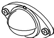
Pilot Lamp indicates whether or not generator is generating electricity, when the engine is driving
