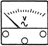
Voltmeter displays the output voltage (Phase to Phase) from the generator.
