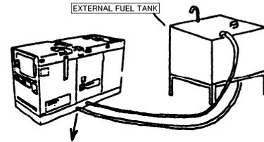
**3** Turn the 3way fuel valve lever to the “B” side.
