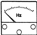
Frequency Meter will display the frequency of the generator. Please check it showing 50Hz during operation.
