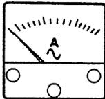
Ammeter displays the output current (Phase) from the generator.
