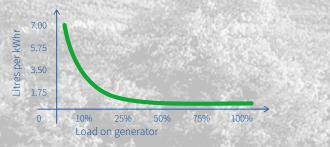
In a hybrid system, the generator only runs when there is work to do. Charging the battery adds to the work, making it burn fuel efficiently. When there is less work to
